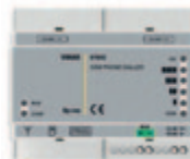
01942 GSM phone dial, for direct connection to Bus 12-24 V~ 50-60 Hz or 12-30 V d.c. (SELV)
