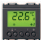
Δ 16921 Thermostat for ambient temperature control (heating and air-conditioning), KNX standard, NO 4 A 24 V~ relay output, 1 input - 2 modules
