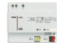
■ 01501 Power supply with Bus 30 V d.c. 640 mA output, 30 V d.c. auxiliary output, supply voltage 230 V~ 50-60 Hz, with decoupling coil, KNX standard
