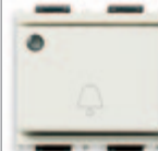
16643.B For emergency call, 2 NO 5 A 250 V~ relay output, supply voltage 12 V~ or 12-24 V d.c. (SELV) - 2 modules
